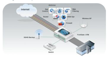
Figure 3 - Connected UTM Secures and Simplifies a Network
