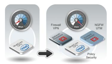
Traditional Security Appliances that use multi- purpose CPU based architectures becomes an infrastructure bottleneck. Even when using multiple multi-core general purpose processors, network security devices cannot deliver the high performance and low latency required.
